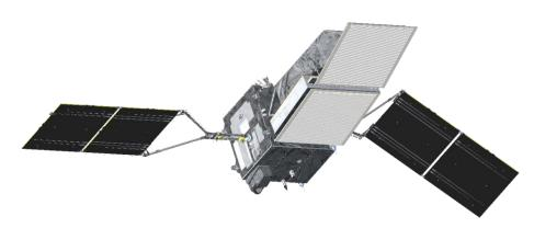
JAXA PMM spacecraft with Ku-band Doppler Precipitation Radar (KuDPR)
